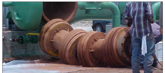
Example of articulated pigs running in excess of 700km through a 36" dry, uncoated pipeline.
