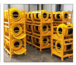
Loading tools can be provided with height - adjustment, mobility wheels and can also be fitted with a winch and cable system to allow removal of pigs from subsea laydown heads and onshore pig receivers.
